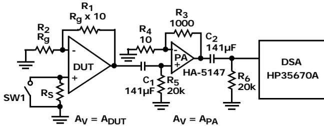
FIGURE 4. COMPLETE LOW NOISE TEST PLATFORM SCHEMATIC
